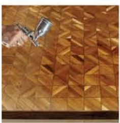
Step-11: Use polyurethane top coats to finish the surface
